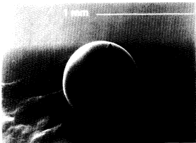
Figure 2 SEM micrograph: A typical polystyrene shell. The shell had been punctured to view the inner surface and wall cross-section
