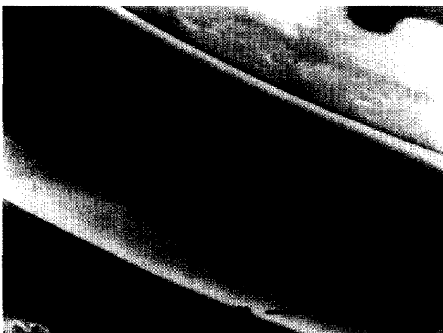
Figure 5 SEM micrographs: Shell wall cross sections. Vacuoles of various sizes appear throughout the wall
